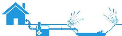
SMALL SEWAGE TREATMENT PLANTS work in a similar way but use powered mechanical parts to aerate the bacteria. This makes them more effective at treating waste water and means they can discharge treated sewage into a soakaway or directly into flowing water.
